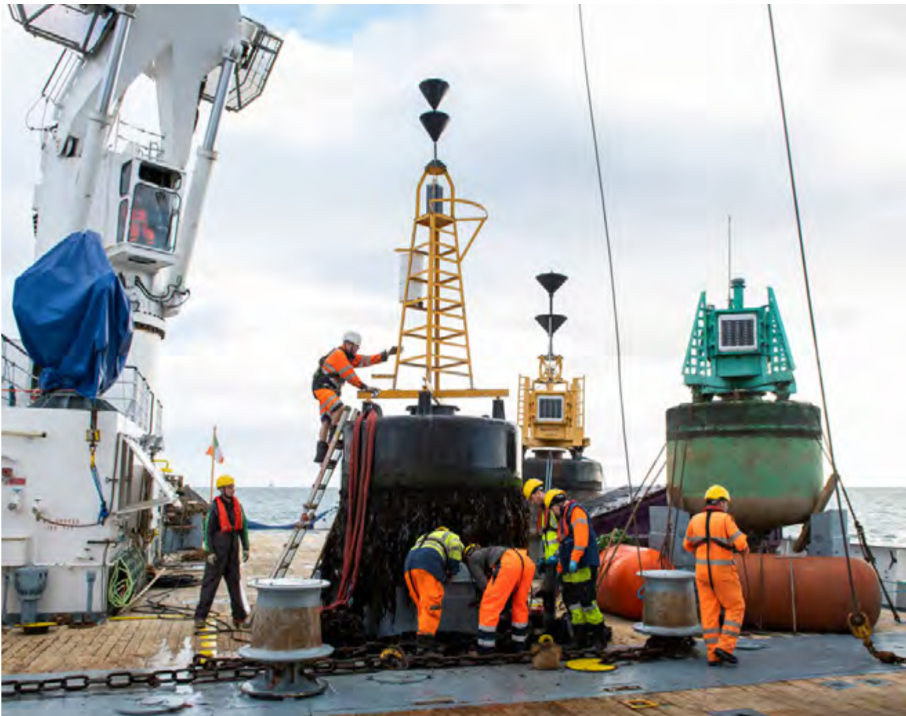
Buoy work on the deck of ILV Granuaile. The ILV Granuaile is equipped with a Class 1 dynamic positioning (DP) technology, which means it can maintain its position and heading with precision, enabling it to operate in some of the most challenging sea conditions found off Ireland's coast. This system allows the vessel and its skilled crew to carry out essential Aids to Navigation operations like buoy and lighthouse maintenance, all year round.
