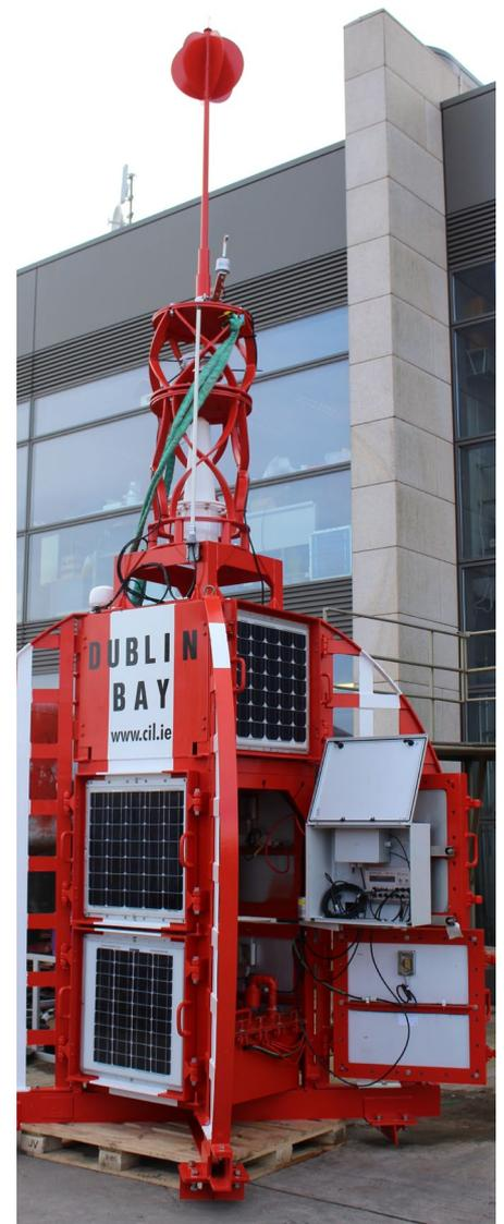
The Dublin Bay Buoy, part of the first phase of the Dublin Bay Digital Diamond e-Navigation Demonstrator, was deployed on the 30th January 2014 and thanks to a suite of sensors is now tweeting met/ocean data available for all users on
